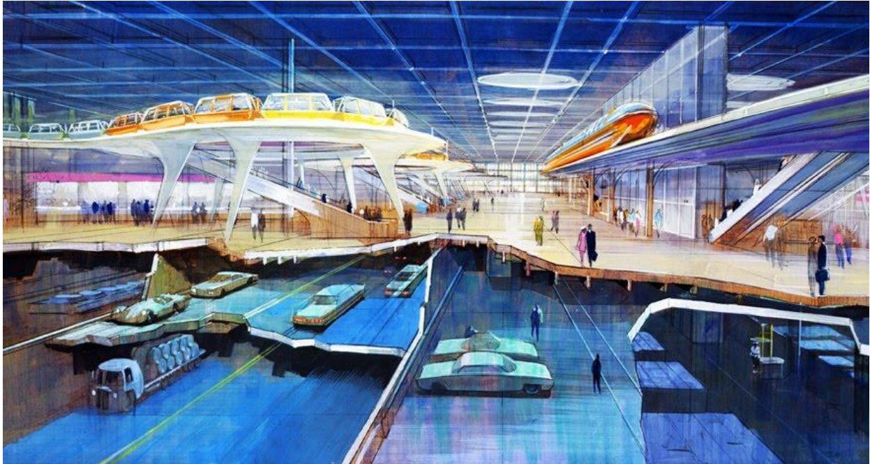
Figure 4. Transit hub located beneath EPCOT's 'urban center', stacking truck and automobile routes, 'WEDWAY People Mover', and monorail tracks vertically (Source: Sklar, 1966)
