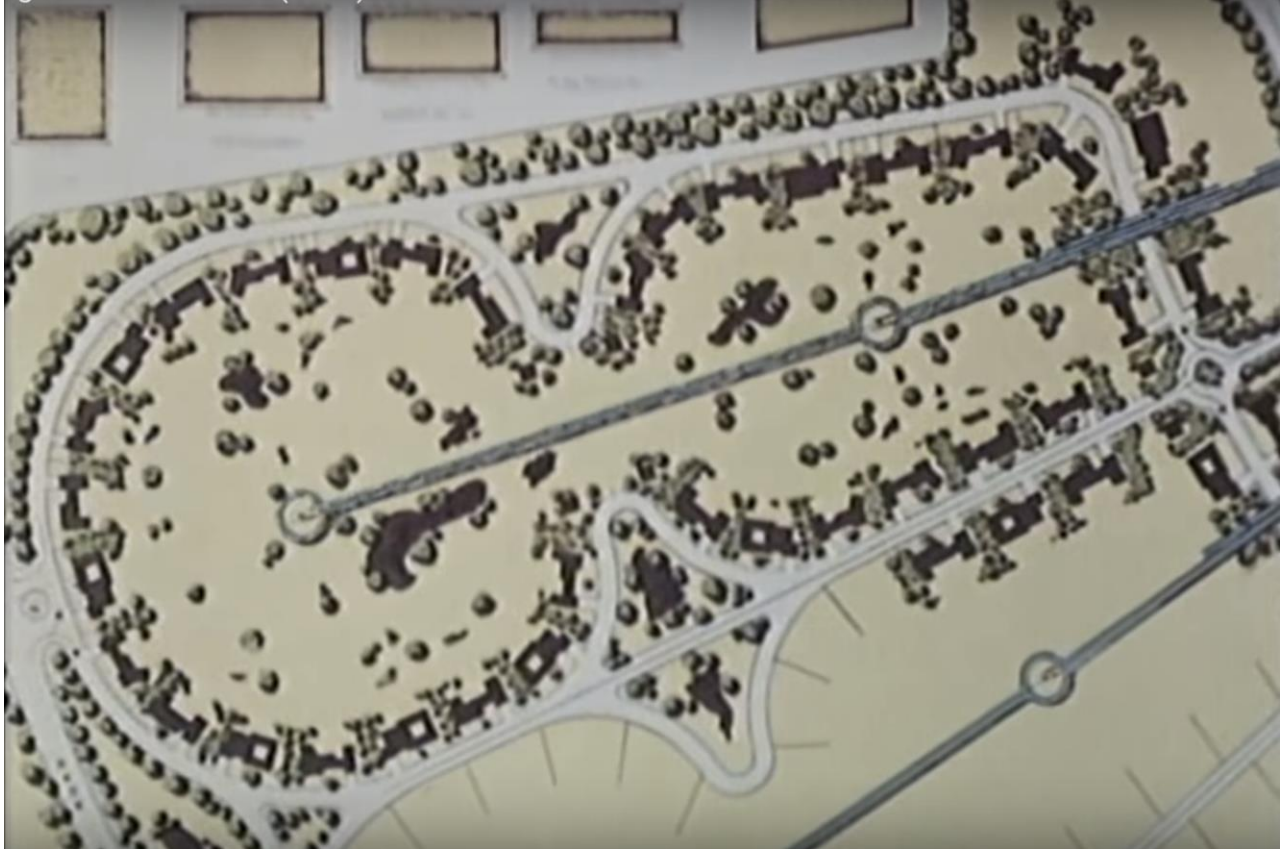
Figure 5. Low-density residential housing superblocks, with 'WEDWAY People Mover' lines and pedestrian-oriented green space separated from automobile traffic (Source: Sklar, 1966)
